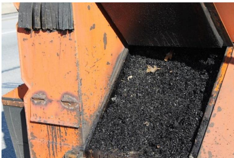
Figure 5.5 Throw-And-Roll Cold Mix Patching Material At I-480
