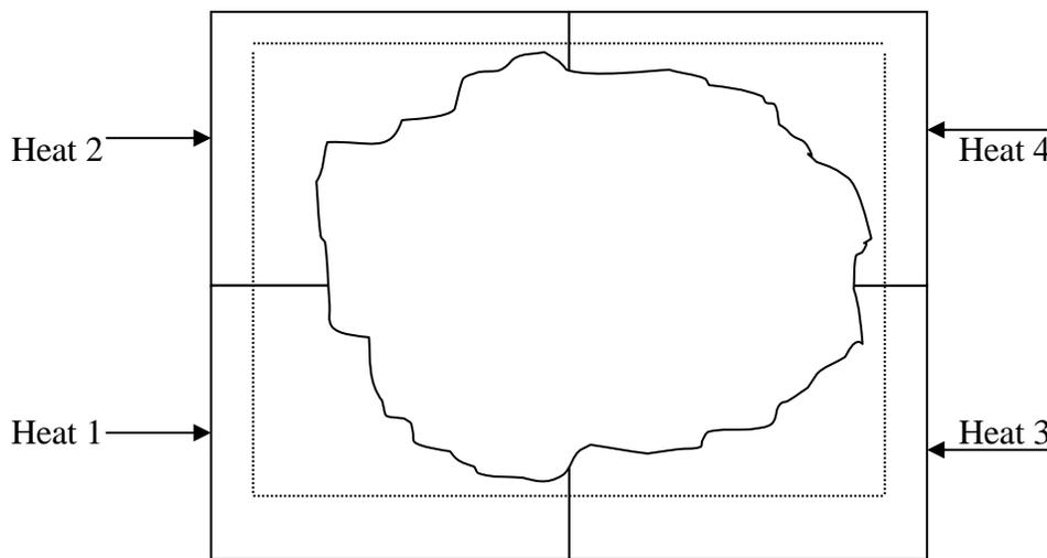
Figure D.2: Multiple Hit Heating Pattern For A Large Repair
