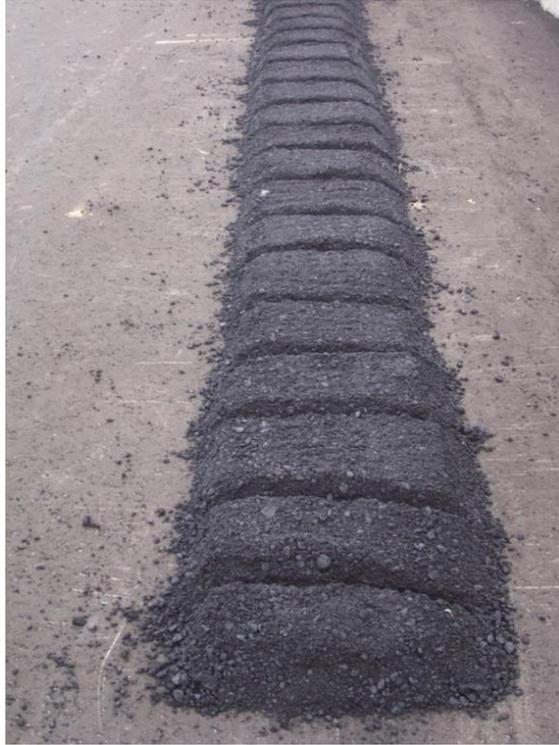
Figure 7.1 Example of Proper Storage Procedure for Asphalt Mixtures Used In Infrared Method
