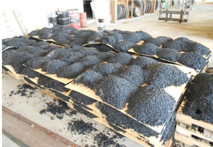
Figure 5.15 Asphalt Patching Materials Stored In Small Piles
