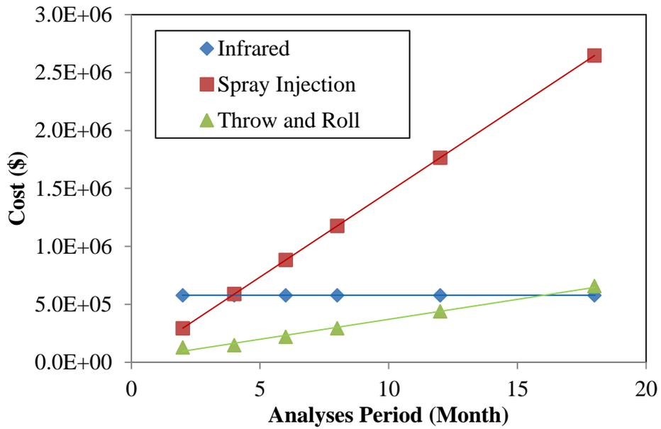
Figure 6.15 Cost of Potholes in District 12 Using Different Analysis Period
