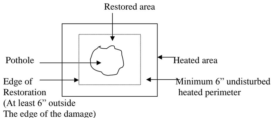
Figure D.1: Proper Heater Placement
