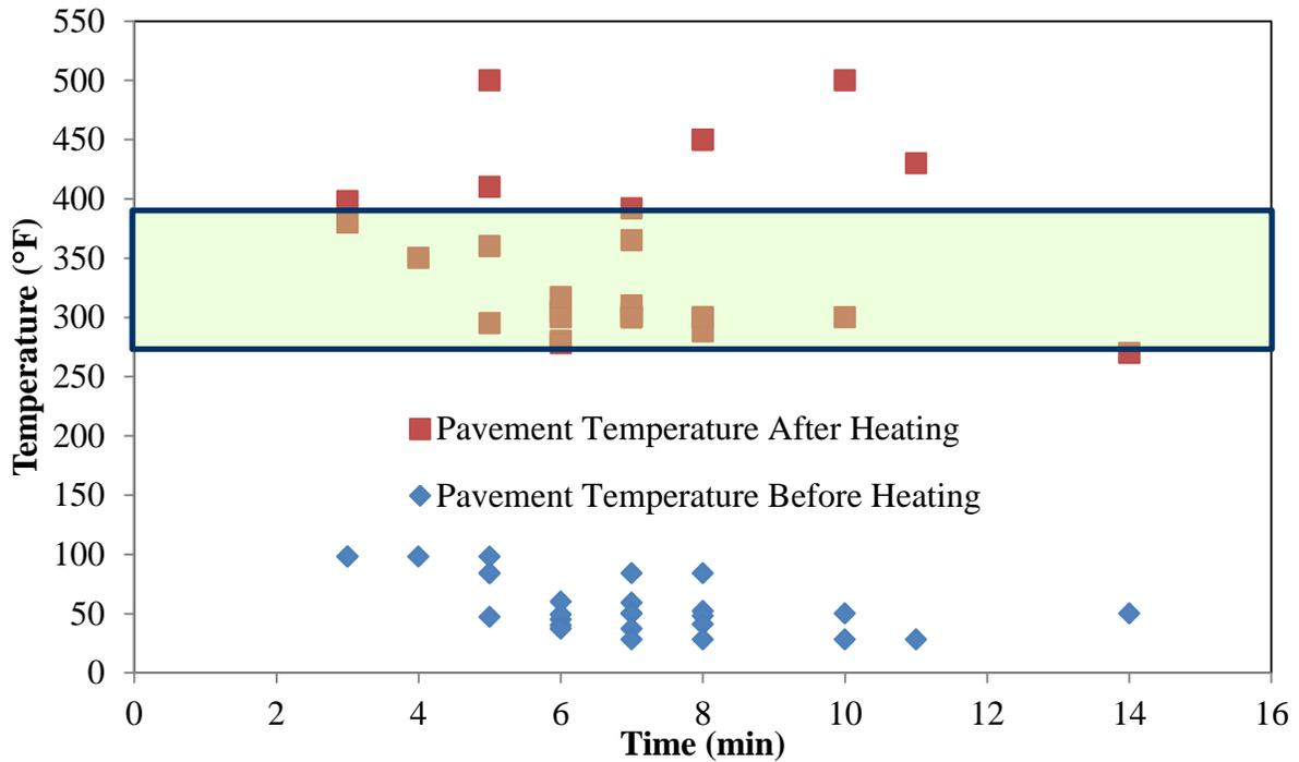
Figure 6.3 Pavement Temperatures Before And After Infrared Heating
