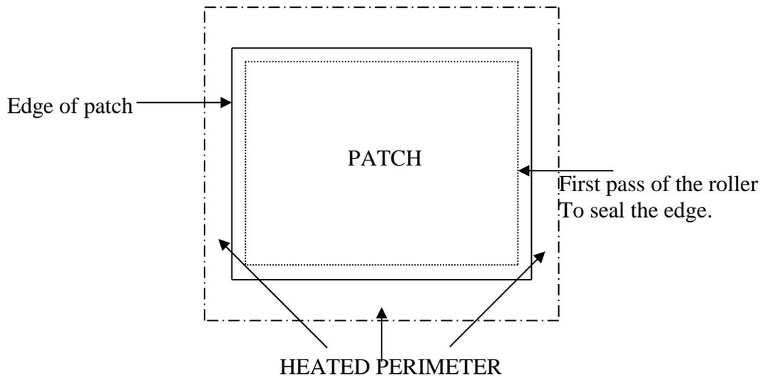
Figure D.3 Demonstration for Proper Compaction Procedure
