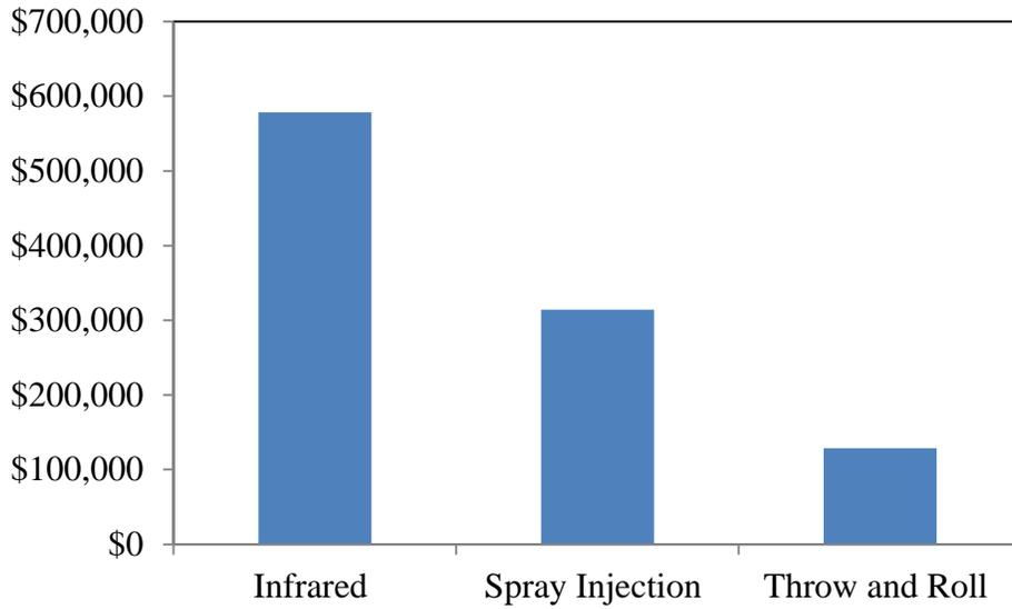
Figure 6.14 Cost of Potholes in District 12 for One time
