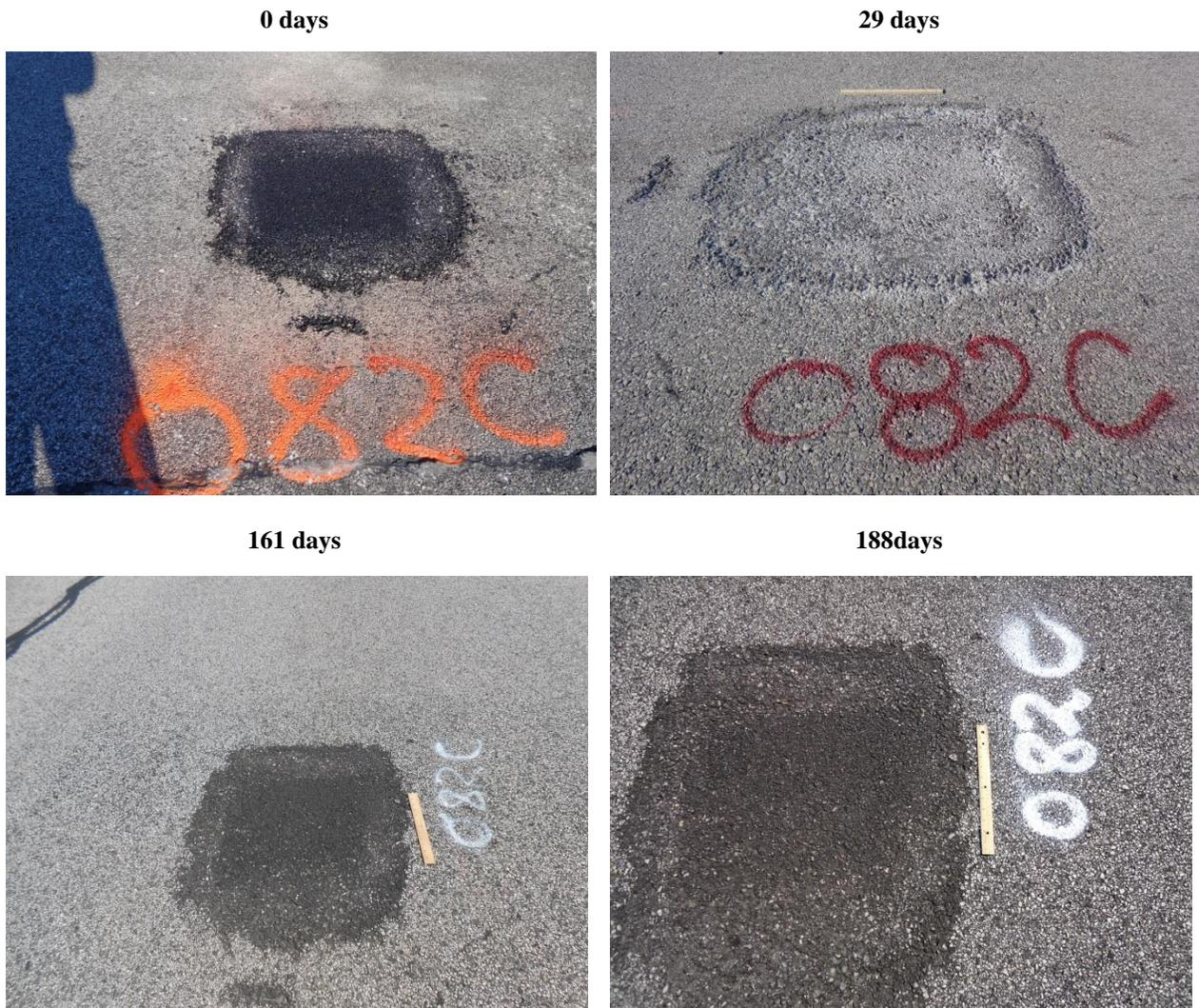
Figure 6.4 Pictures for Infrared Patch after 0, 29, 161, And 188 Days Of Installation
