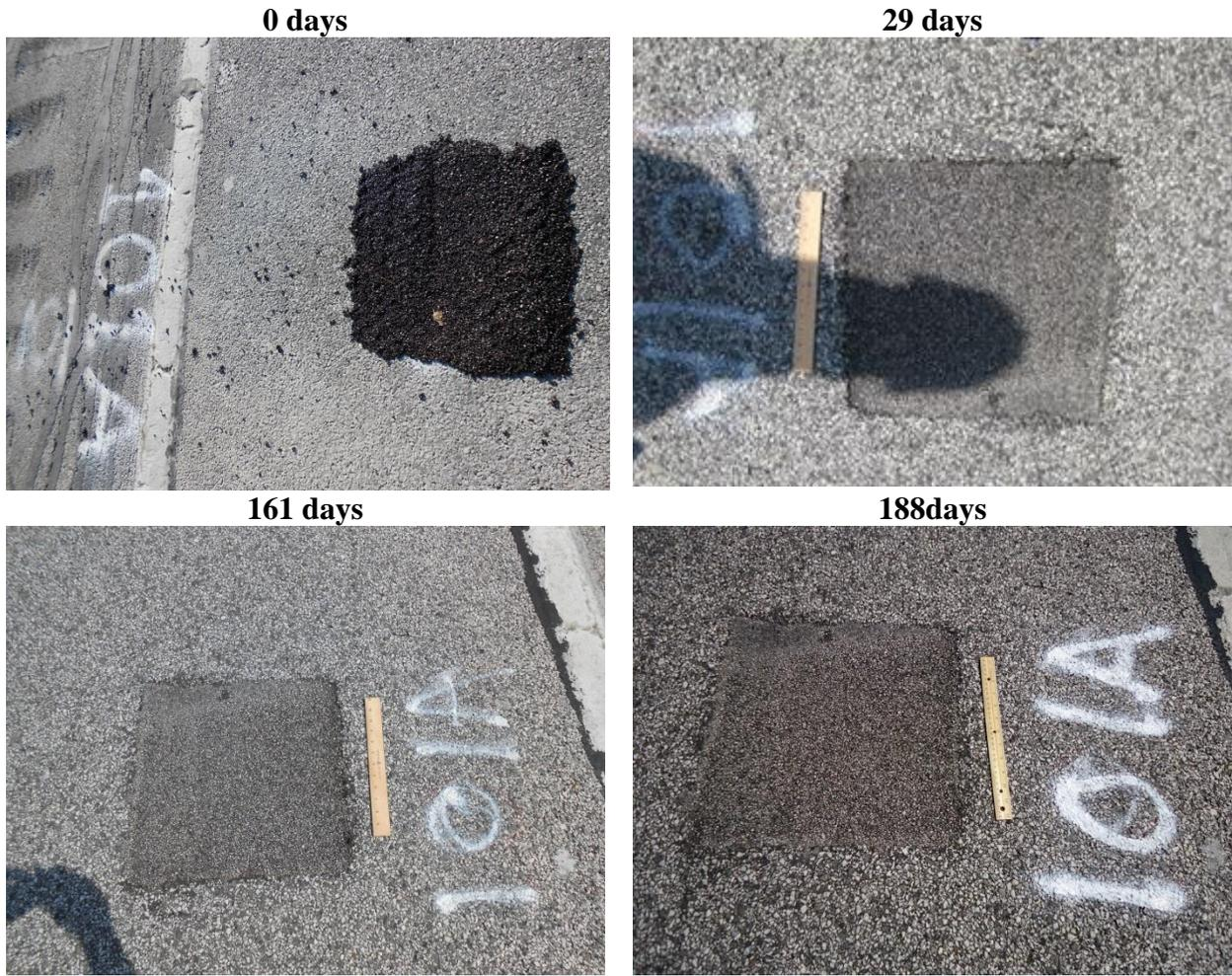
Figure 6.6 Pictures for a Throw-and Roll Patch after 0, 29, 161, And 188 Days Of Installation
