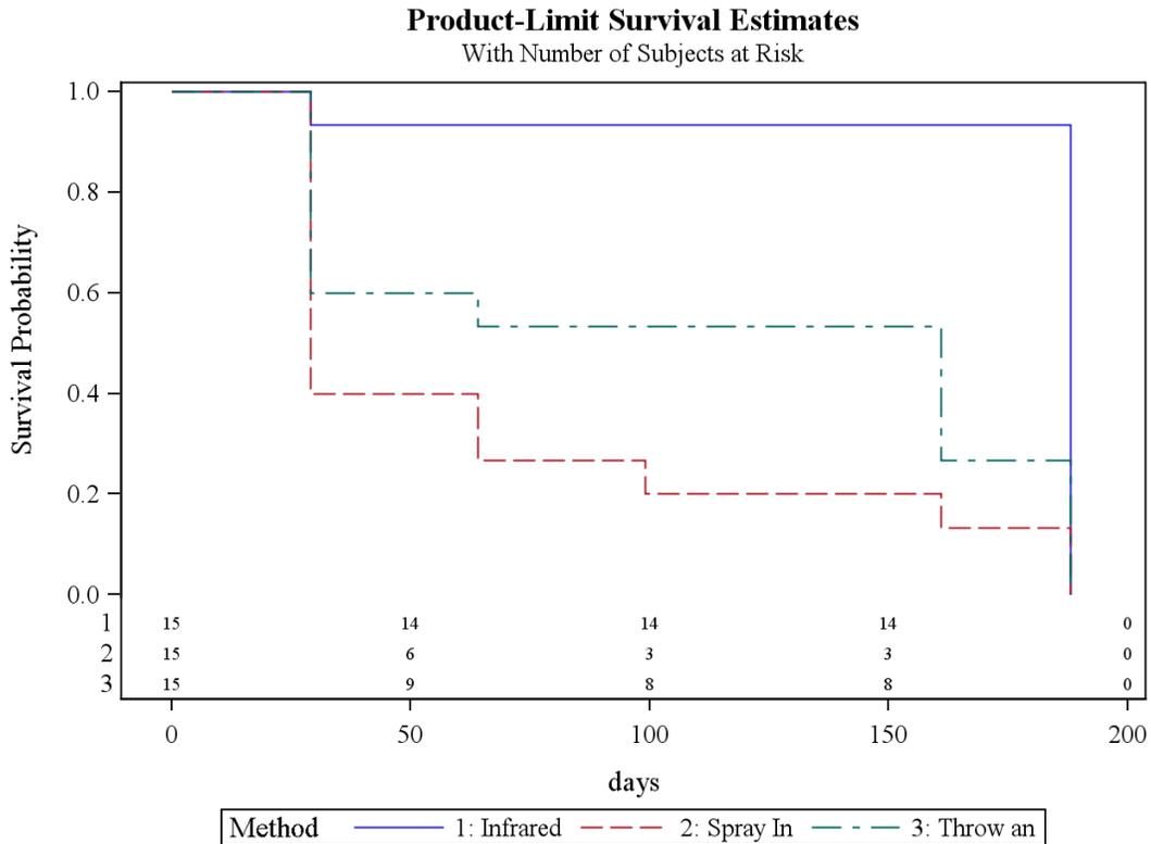
Figure 6.13 Survival Curves For The Different Patching Methods
