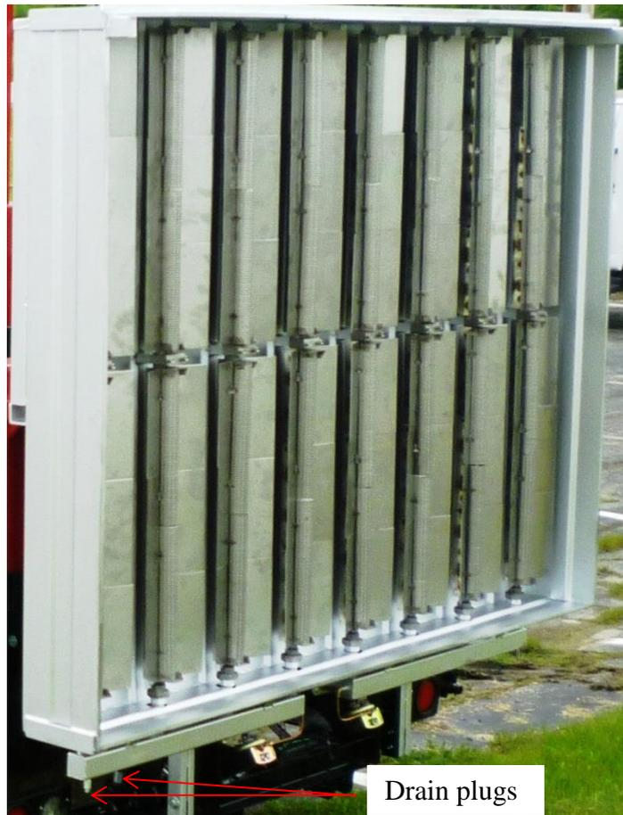
Figure 5.9 Drain Plug at the Bottom Of Each Manifold In The Infrared Heater
